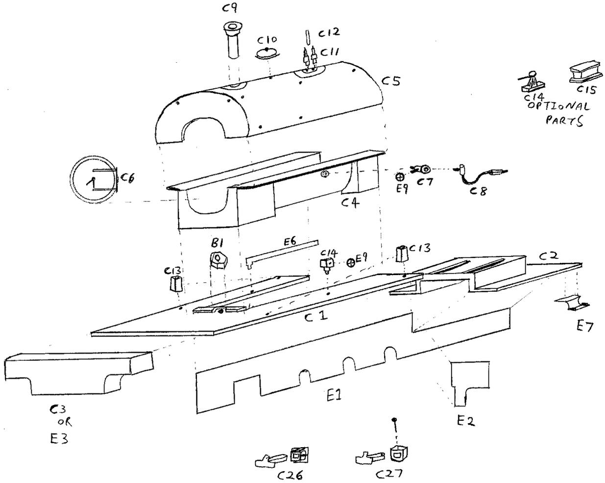
Fig3. Cab construction
