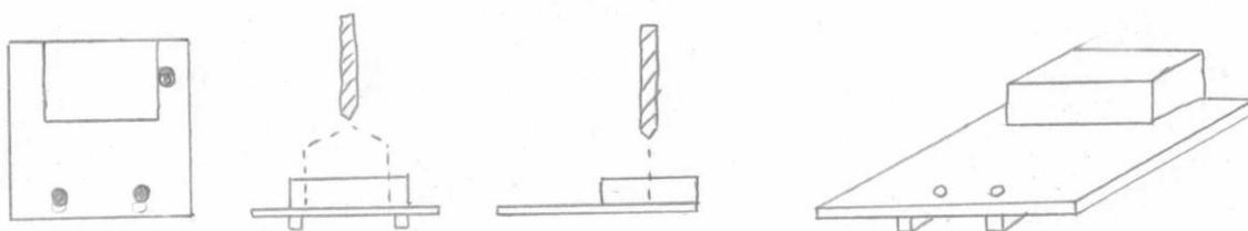
GUIDE FOR DRILLING ADDITIONAL HOLES ON CAB
